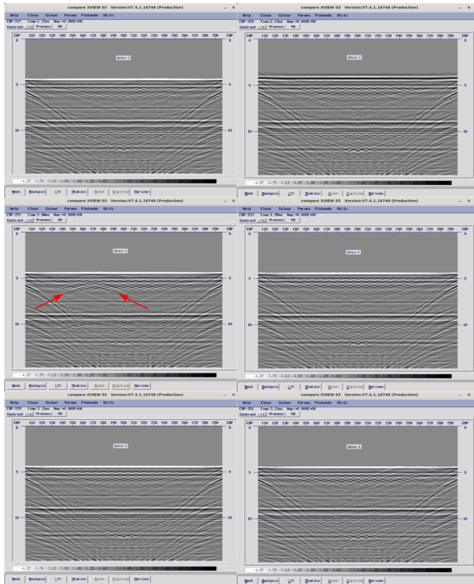
Figure 24. Stacked section for the six defects. Only Defect 3 (middle-left) has a clear diffraction response (red arrows). Same scaling has been applied to all sections.
