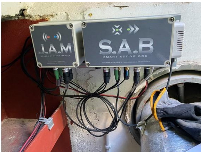
Figure 3. Measurements performed with acoustic sound waves (Delta-T) (photo Öresundskraft).
