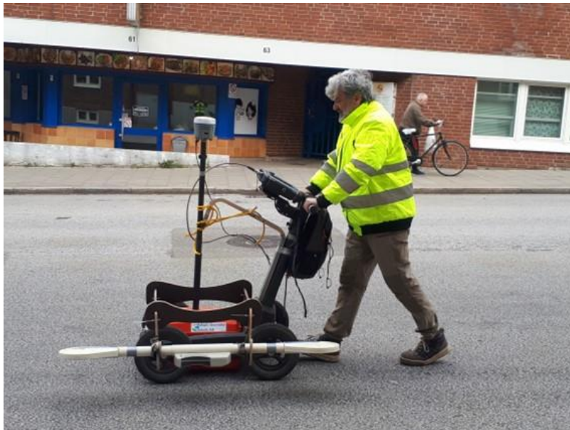
Figure 2. Measurements carried out with georadar technology (photo Öresundskraft).
