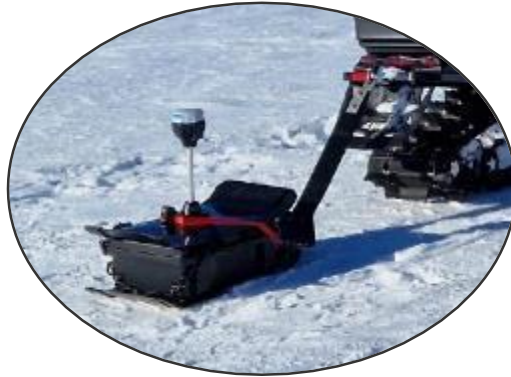
RTK rover on snow mobile sled
