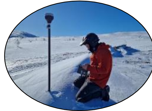
RTK base station
