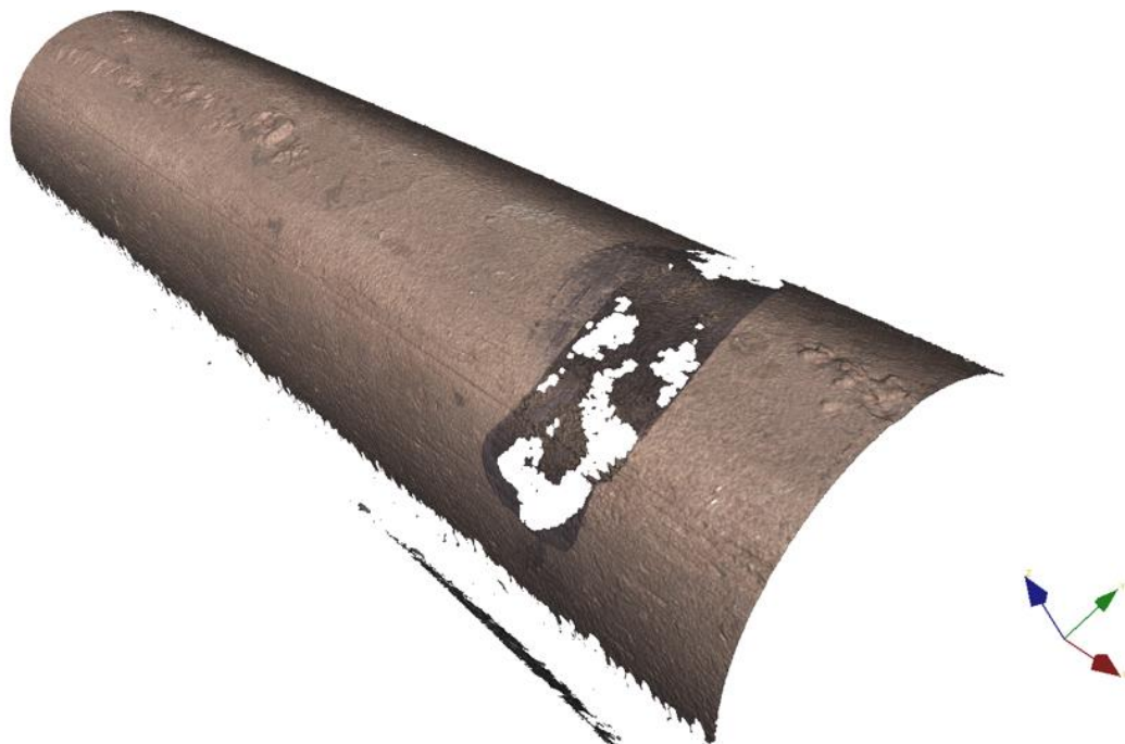
Figur 90: Prov 11 – Inre karded. Grotdjup 1-2 mikrometer.
