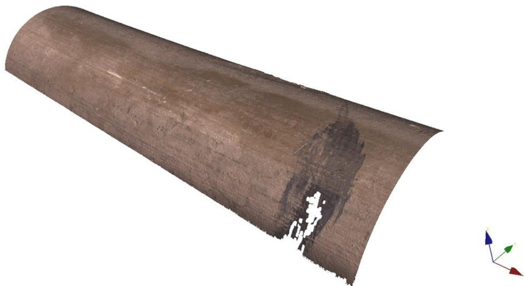
Figur 81: Prov 7 – Inre karded. Gropdjup 1-2 mikrometer.
