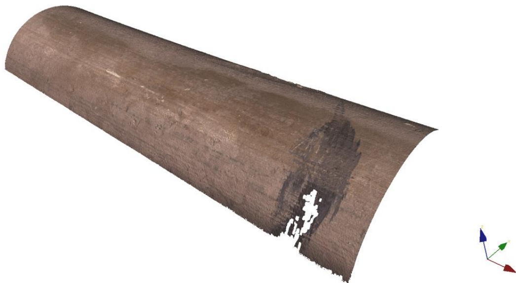
Figur 81: Prov 7 – Inre karded. Gropdjup 1-2 mikrometer.
