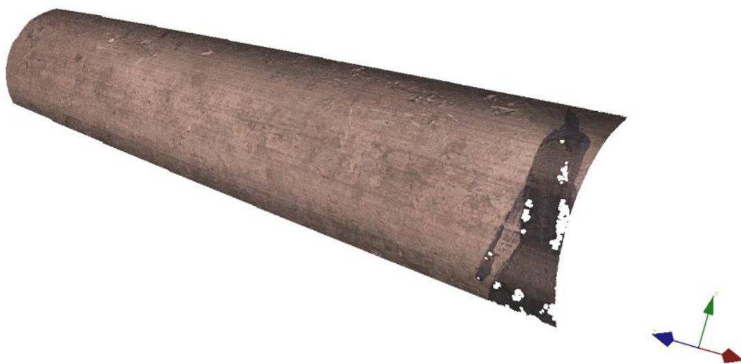
Figur 68: Prov 2 – Inre karded. Grotdjup 28 mikrometer.
