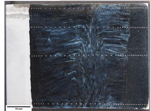
Double-buttering repair weld
