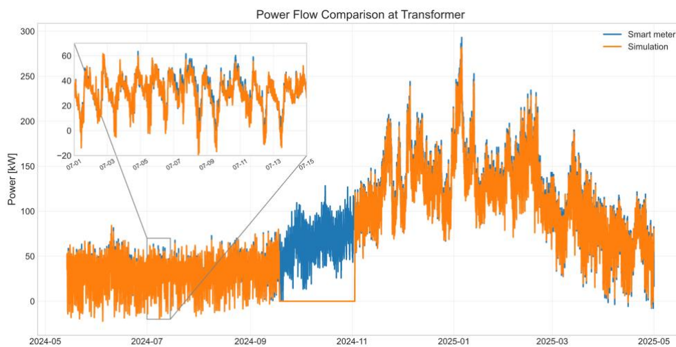
Figure 6: Comparison between measured and simulated transformer power flow. Simulation is missing 18/09/2024 – 02/11/2024 due to the missing data in analytics logs.
