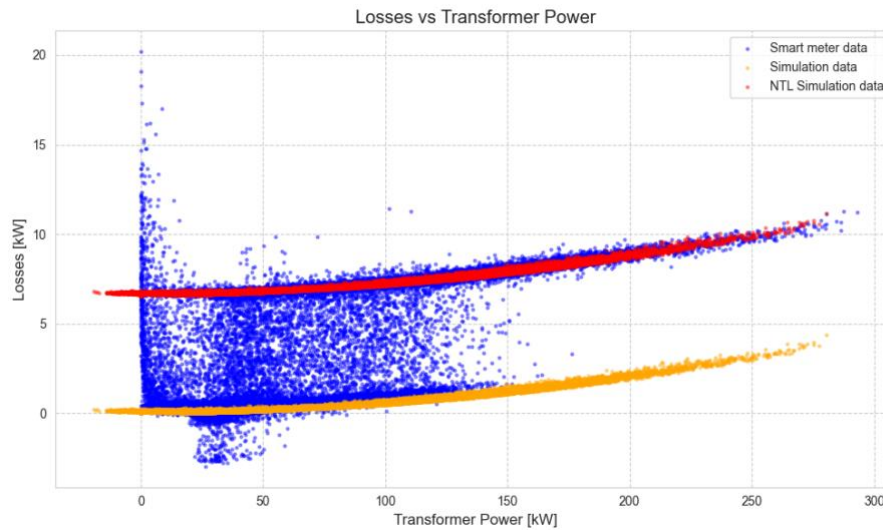
Figure 8: Comparison of losses between measurement, simulation and simulation with additional NTL-load.
