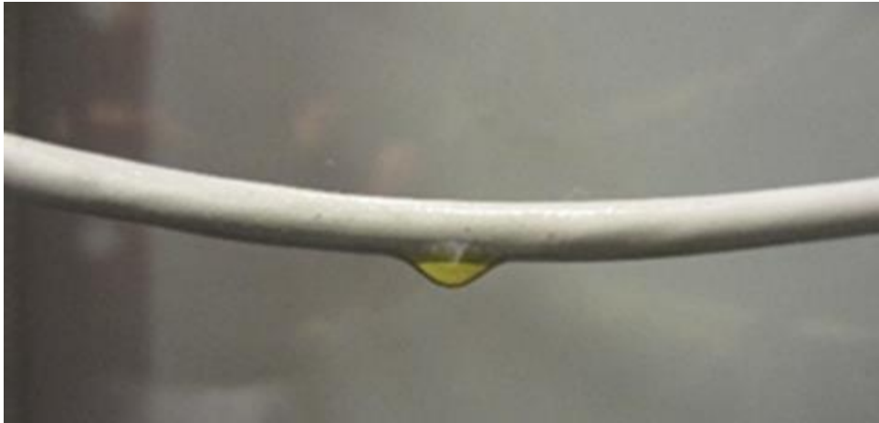
Figure 2. Photo provided by the nuclear power plant which captures the observation of the plasticizer coming out of the cables during service
