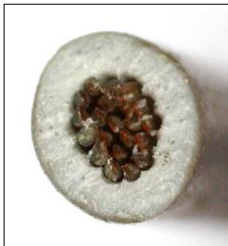
Figure 8. The cross section of the 0.75 mm 2 cable which had been post-aged for 2159 hours.
