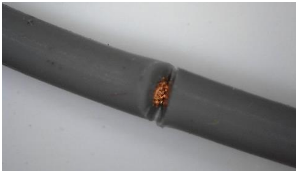
Figure 9. Cutting a new fresh cross section in the 0.5 mm 2 cable post-aged for 2159 hours.
