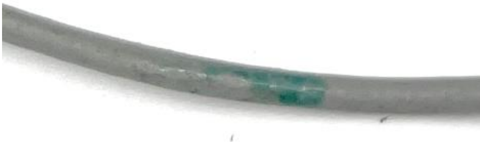
Figure 6. Enlarged view of one of the 0.75 mm 2 cables showing the green sticky deposit that was found to a lesser degree on these cable strands compared to the 0.5 mm 2 .
