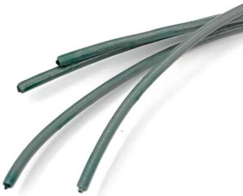
Figure 4. A close-up of the photo in Figure 3 showing the end section of the 0.5 mm 2 cable strands post-aged for 2159 hours at 75°C
