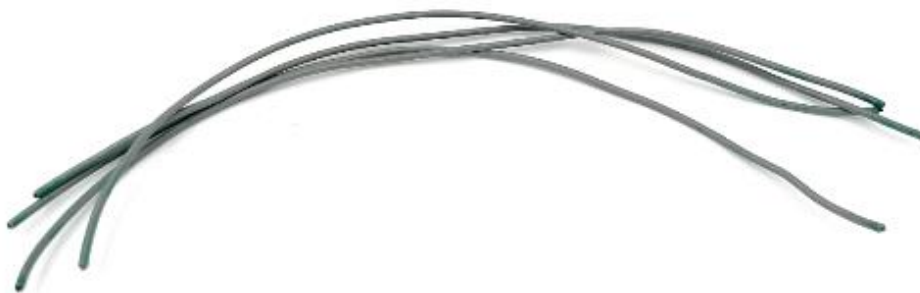
Figure 3. A photo of the 0.5 mm 2 cable strands post-aged for 2159 hours at 75°C
