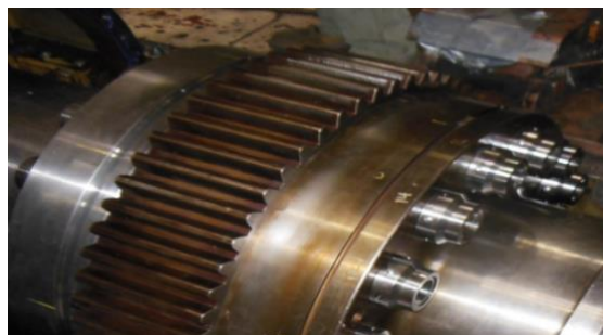
Figure 28 Coder Based Measurement by means of Gear Teeth and Magnetic Pick Up
