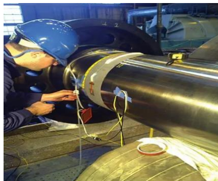
Figure 24 Mounting and Fixing of the Sensors on the Shaft Surface
