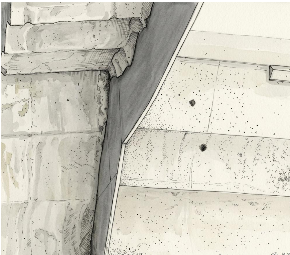
Figure 16. Schematic illustration of gap formation observed in Swedish containment walls during opening of the reactor wall. The inner containment wall is shown on the left-hand side, where a gap is present between the steel liner and the inner concrete wall.
