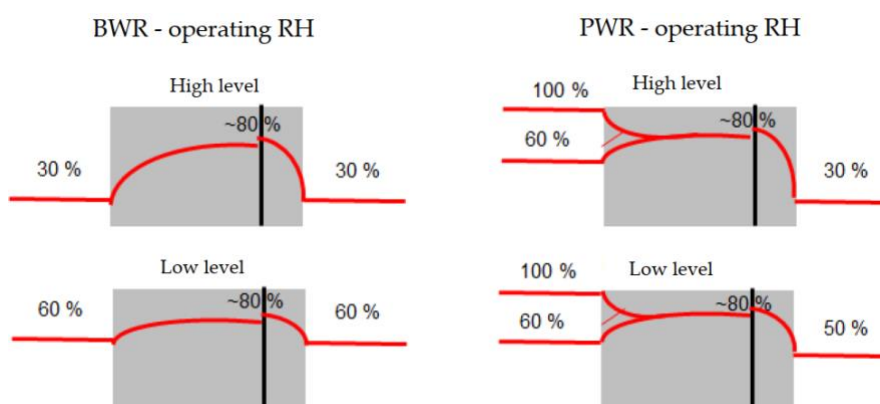
Figure 9. Relative humidity in the cylindrical wall and the surrounding spaces in BWR and PWR during operation (Sandberg et.al., 2019).
