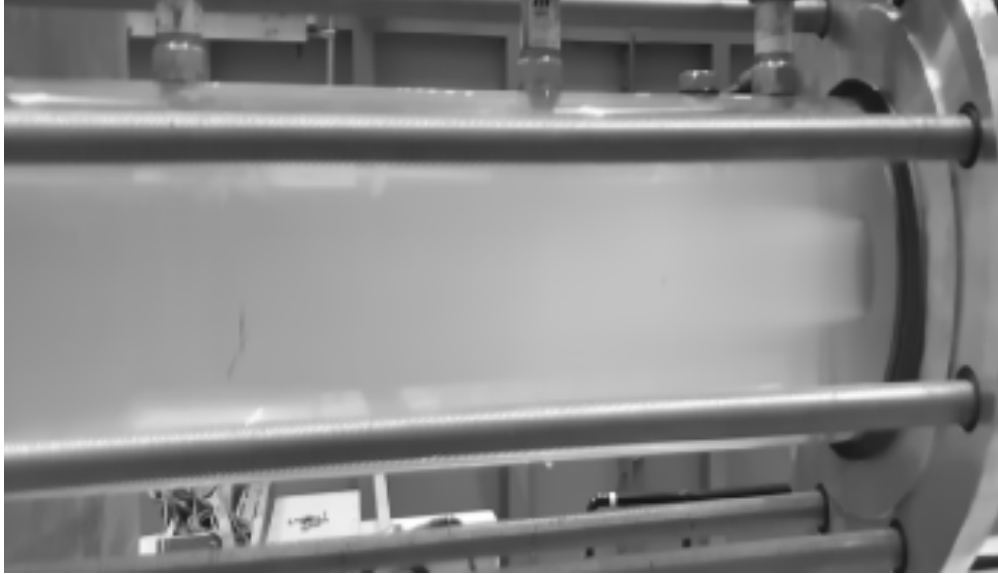
Figure 7. Mean cavitation field for the single-hole orifice plate.
