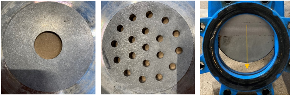
Figure 3. The single-hole orifice plate with a centered d=32 mm hole, the multi-hole orifice plate with 19 evenly distributed holes with diameters of 7.2 mm and 7.4 mm (two different plates) and the adjustable Stafsjö valve with an adjustable plate perpendicular to the flow.
