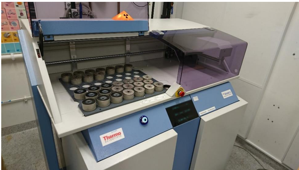
Figure 22 The testing setup for X-ray fluorescens measurements of elements content in steel.
