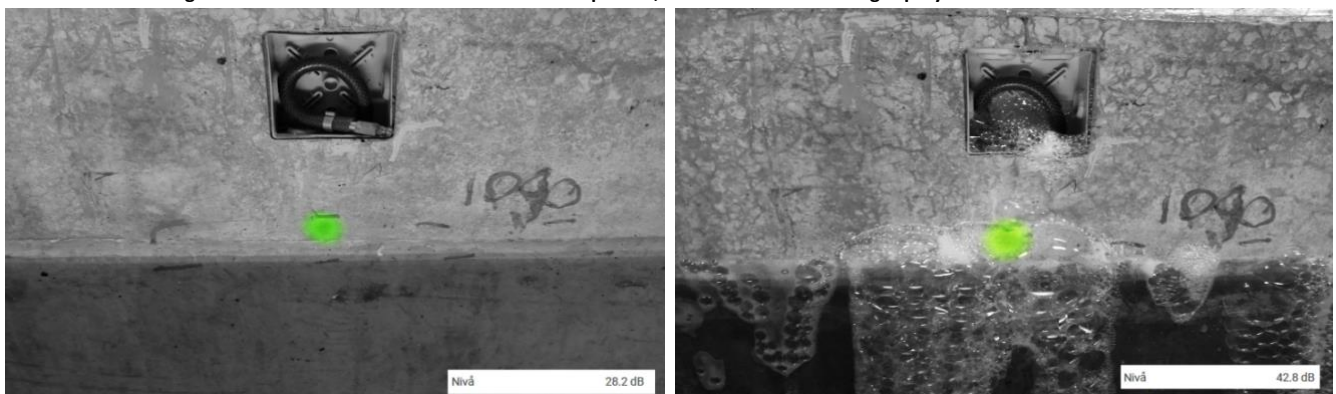
Figure 11 Pictures from NL ACOUSTICS at reference point 2, without and with leakage spray.
