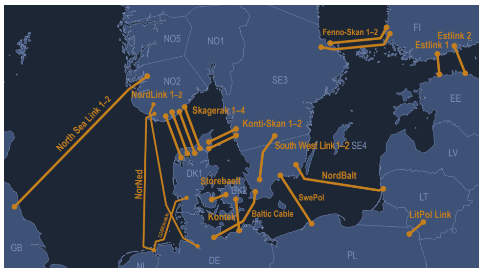
Figure 1-1 HVDC links in the Nordic synchronous system [2]. Note that the HVDC links LitPol Link and COBRA cable shown in the figure are not within the Nordic synchronous system.
