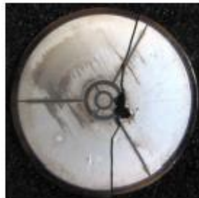
Figure 4-5 Defective thyristor - module SSW2 TH2
