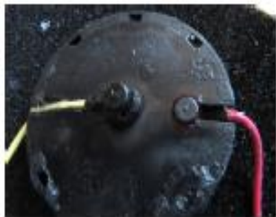
Figure 4-6 Faulty cathode spring
