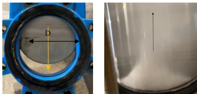
Figure 1. The flow and cavitation through an almost fully closed knife gate valve.
