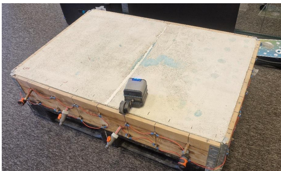
Figure 21 - Test block at the supplier's site with two layers of rebar.
