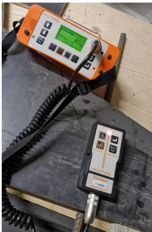
Figure 12 - Sensor placed directly above the rebar and aligned in the same direction as the bar.
