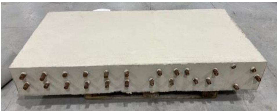
Figure 2 - The same test block after casting, surveyed with GPR and ultrasound.
