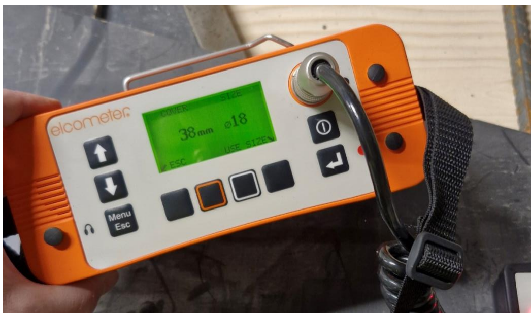
Figure 13 - Example of the instrument's estimated rebar diameter function. In this example, the instrument detected 38 mm to a \varnothing 18 bar instead of the actual 40 mm to a \varnothing 16 bar.
